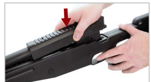
With outer barrel positioned correctly at the front, press down by the trigger assembly to seat it.
